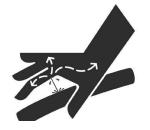
Escaping fluid under pressure may penetrate the skin causing serious injury. Avoid the hazard by relieving pressure before disconnecting hydraulic lines. Tighten all connections before applying pressure and inspect hoses regularly for wear or damage. If an accident occurs, see a doctor immediately. Any fluid injected into the skin must be surgically removed within a few hours or gangrene may result.
