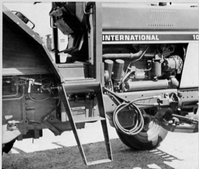
Installation Kit Model IHK-86 installed on tractor ready for sprayer plumbing.
